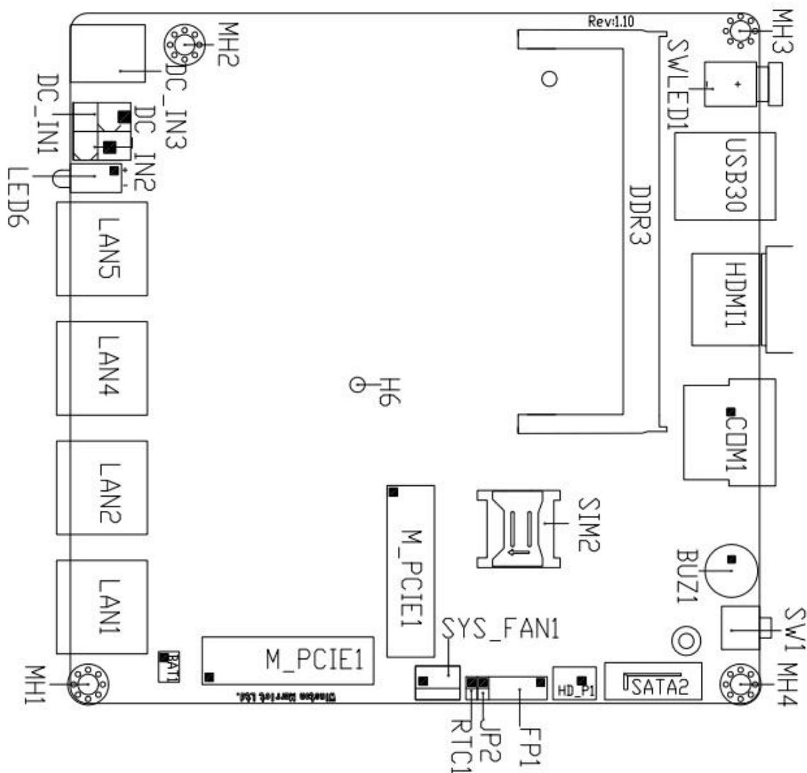
Note: The interface in the figure, the pin is square and is Pin 1.
