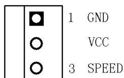
CPU fan interface, support automatic speed adjustment. The maximum voltage of the fan is equal to the input power supply voltage. When the input power supply voltage is high, be careful to select the appropriate fan. The SYS fan does not support automatic speed adjustment.
