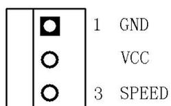
CPU fan interface supports automatic speed adjustment. The maximum voltage of the fan is equal to the input power supply voltage. When the input power supply voltage is high, please pay attention to choose the appropriate fan. SYS fans do not support automatic speed adjustment.
